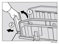
4 Lower or lift the paper alignment wings .
